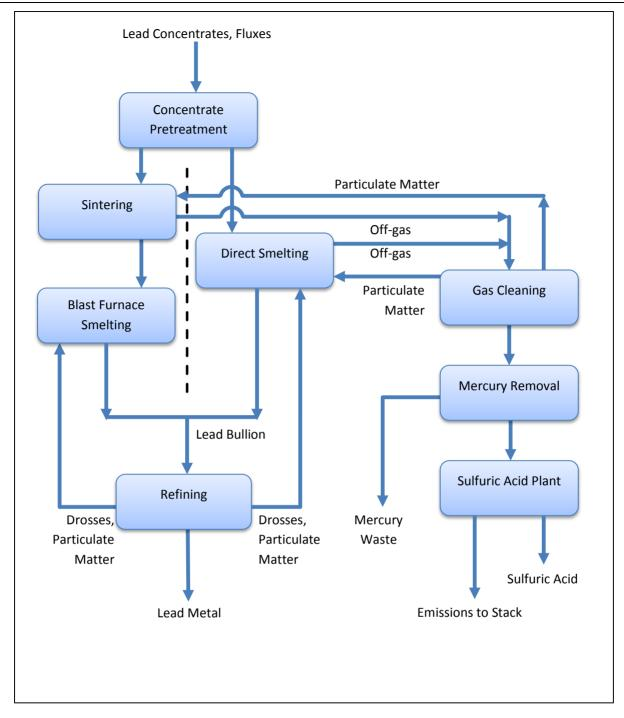
Figure 1. Processes in primary lead production
