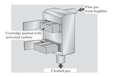
Figure 1. Activated carbon adsorber
