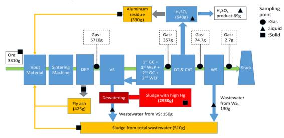
*Key*: DEP: dry electrostatic precipitator, VS: Venturi scrubber, GC: gas cooler, WEP: wet electrostatic precipitator, DT: dehydration tower, CAT: converting process and absorption tower, WS: wet scrubber
