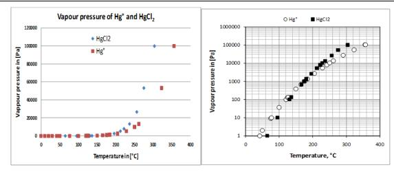
Figure 6.2. Dependence of the vapour pressure of Hg° and HgCl<sub>2</sub> on the temperature (left chart with linear scale and right chart with logarithmic scale) (Holleman-Wiberg, 1985; CRC Handbook, 1976; CRC Handbook, 1995; CRC Handbook, 2012)
