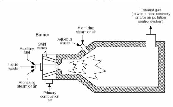
Figure 3 Typical liquid injection incinerator
