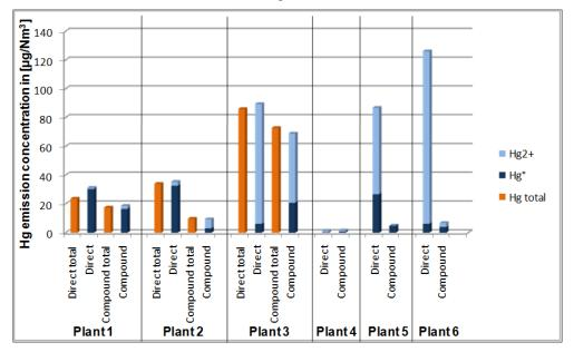
Figure 6.10. Emissions to air of elemental and oxidized mercury according to different sources Indications for the sources of data: Plant 1 and plant 2: Oerter/Zunzer, 2011 Plant 3: VDZ Activity Report, 2002
