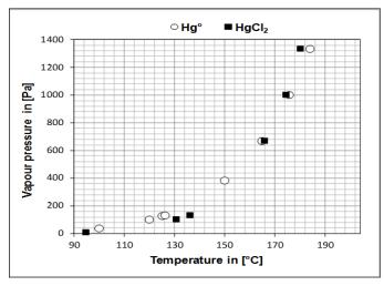
Figure 6.5. Dependence of the vapour pressure of  $Hg^{\circ}$  and  $HgCl_2$  on the temperature between 90 °C and 190 °C (Schoenberger, 2015)
