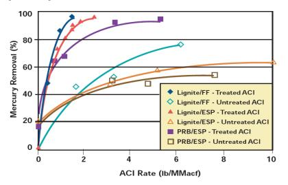
Figure 10. Comparison of untreated activated carbon and treated activated carbon performance for mercury removal
